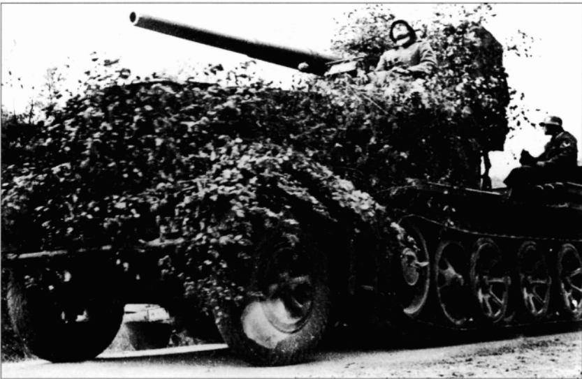
Something the Panzer Division greatly missed in 1940: a heavy, self-propelled, anti-tank gun. Apart from the Panzerjäger I, built on the PzKpfw I chassis and armed with a Czech 47mm gun, there was only one other self-propelled AT gun available: the 88mm Flak 18 (sfl) auf Zugkraftwagen 12t SdKfz 8. Twenty-five examples of this vehicle were produced in 1939/40 to provide German Army units with a heavy anti-tank SP gun also capable of dealing with enemy fortifications. They were used to equip 8. schwere Panzerjäger Abteilung.
