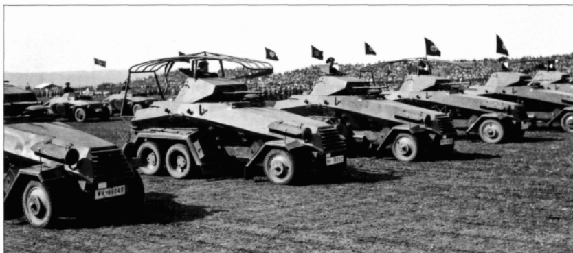
Six-wheeled SdKfz 231 armoured cars on parade in a training ground, probably in 1935. Based on the chassis of the Krupp 'Protze' L2H143 Kfz 81 2.6-ton light lorry, 123 examples were produced between 1932 and 1937 and were used to equip the heavy platoons of the Panzerspäh Kompanien. Due to its limited off-road mobility, it was withdrawn from frontline service after the French campaign.
