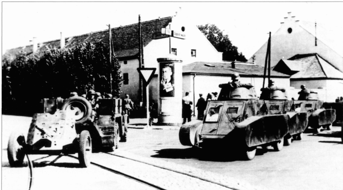
The Panzerwaffe in its infancy: Panzer-Attrappe (dummy tanks) conduct training with anti-tank guns, in this case the 37mm Pak 35/36. Initially made of wood and later of light steel alloy, these dummy tanks were mounted on cars. Their purpose was to get soldiers and tank crews acquainted with cooperating with armoured vehicles.
