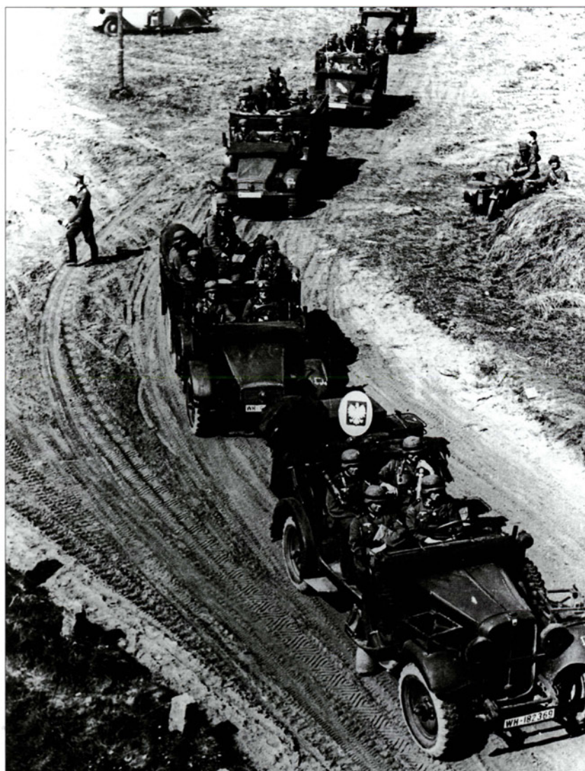
A column of Krupp L2H143 Kfz 81 2.6-ton light lorries, commonly used to carry half a Schützen or a machine-gun squad, led by a Horch 830 Kfz 15 communication car on a march in the early stages of the Polish campaign. The tactical symbol on the left mudguard denotes a motorized infantry platoon.
